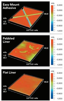
Microscopic view of adhesive surface measured with interferometer.
