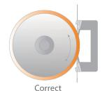
**PROPER SYSTEM ALIGNMENT** For consistent ink metering, best print quality and optimized blade life, an enclosed chamber system requires perfect alignment (both horizontal and vertical) so that both blades have equal amounts of pressure. Incorrect alignment creates uneven blade pressure, blade wear and/or ink leakage.
