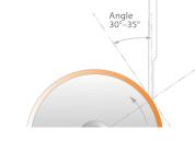
**REVERSE ANGLE DOCTOR BLADES** Provide excellent printing and wiping. To obtain best results, the blade holder must be cleaned carefully and be in good condition. The Doctor Blade must be mounted absolutely straight and without waves. To prevent waves, tighten bolts in the blade holder from the center out. As always, minimal pressure is the key to successful printing.
