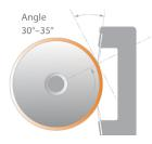
**CHAMBER DOCTOR BLADE SYSTEMS** There are two distinctly different blade systems; single Reverse-Angle Blade system and the more commonly used Enclosed Doctor Blade System. Angles on an enclosed system are pre-set and for single reverse-angle blade system the industry standard is approximately 30 to 35 degrees. Flat angles create greater contact area, requiring more doctor blade pressure to get a clean wipe. This increase in pressure creates excessive anilox and blade wear.
